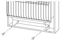
Figure 11 - Installing Bottom Mounting Screws
